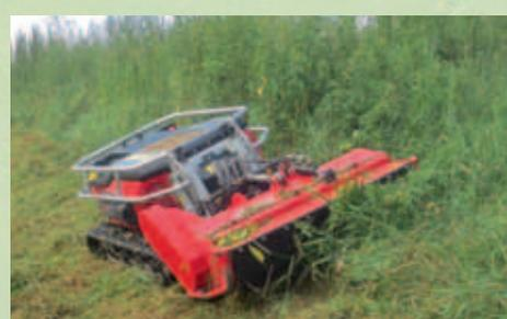
The tracks are independently suspended allowing 4 points of ground contact at all times.
