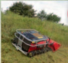
With its low point of gravity the Timan RC-1000 works safely on slopes of up to 50° - without any problems...
